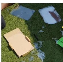
Cutting jig to ensure accuracy and consistency when cutting the face shield part.
