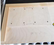
Drilling Jig to ensure accuracy of where the holes in the visors go.
