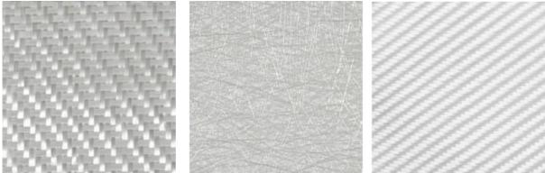
The pattern of weave determines the strength and weight of the Glass Reinforced Plastic, after resin has been added. Different weaves have been developed for different practical applications.
